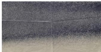
(g) Fabric 5: The edges are darker than the middle which indicates a pressure drop in the spraying system
