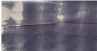
(e) Fabric 3: The alternating between a lighter and a darker colour indicates that there probably has been a pressure drop in the spraying system.
