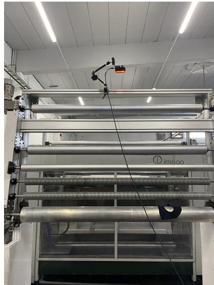
Figure 9: Camera setup when taking pictures of fabric in the real machine. The fabric is moving through the top cylinder
