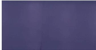
(d) Fabric 2: The colour of the fabric is a different colour shade than the correctly dyed fabric as well as the lines that are lighter.
