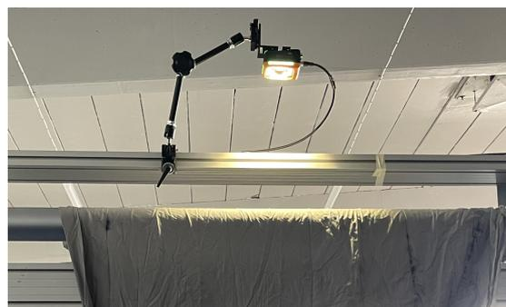
Figure 10: Camera taking picture of fabric lying still. The fabric is lying still on the cylinder to simulate the real machine when standing still
