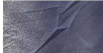
(c) Fabric 1: The darker colour on the right side indicates that the nozzle is partially clogged and will spray unevenly
