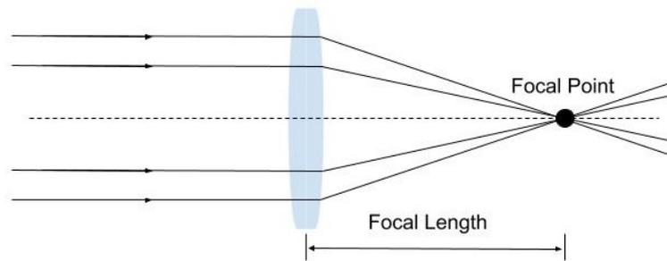
Figure 2: Focal length and focal point related to the incoming light and lens
