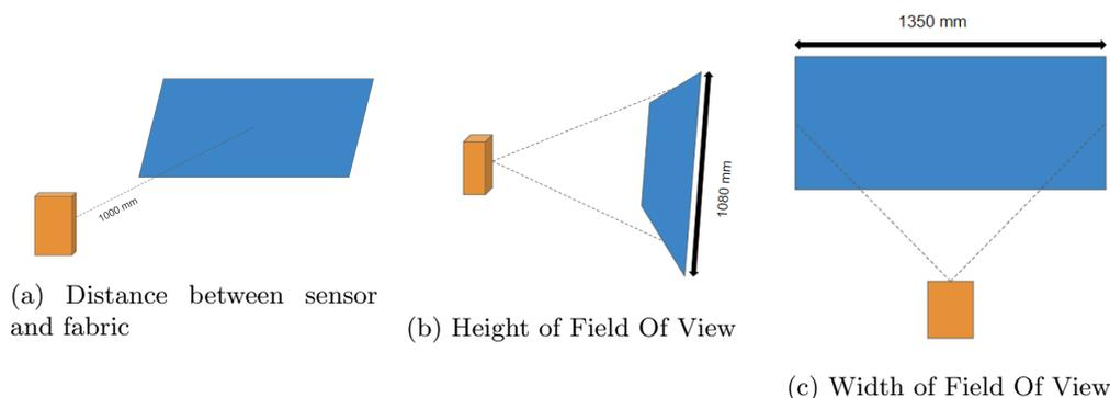
Figure 16: Illustration of sensor setup showing installation distance and FOV
