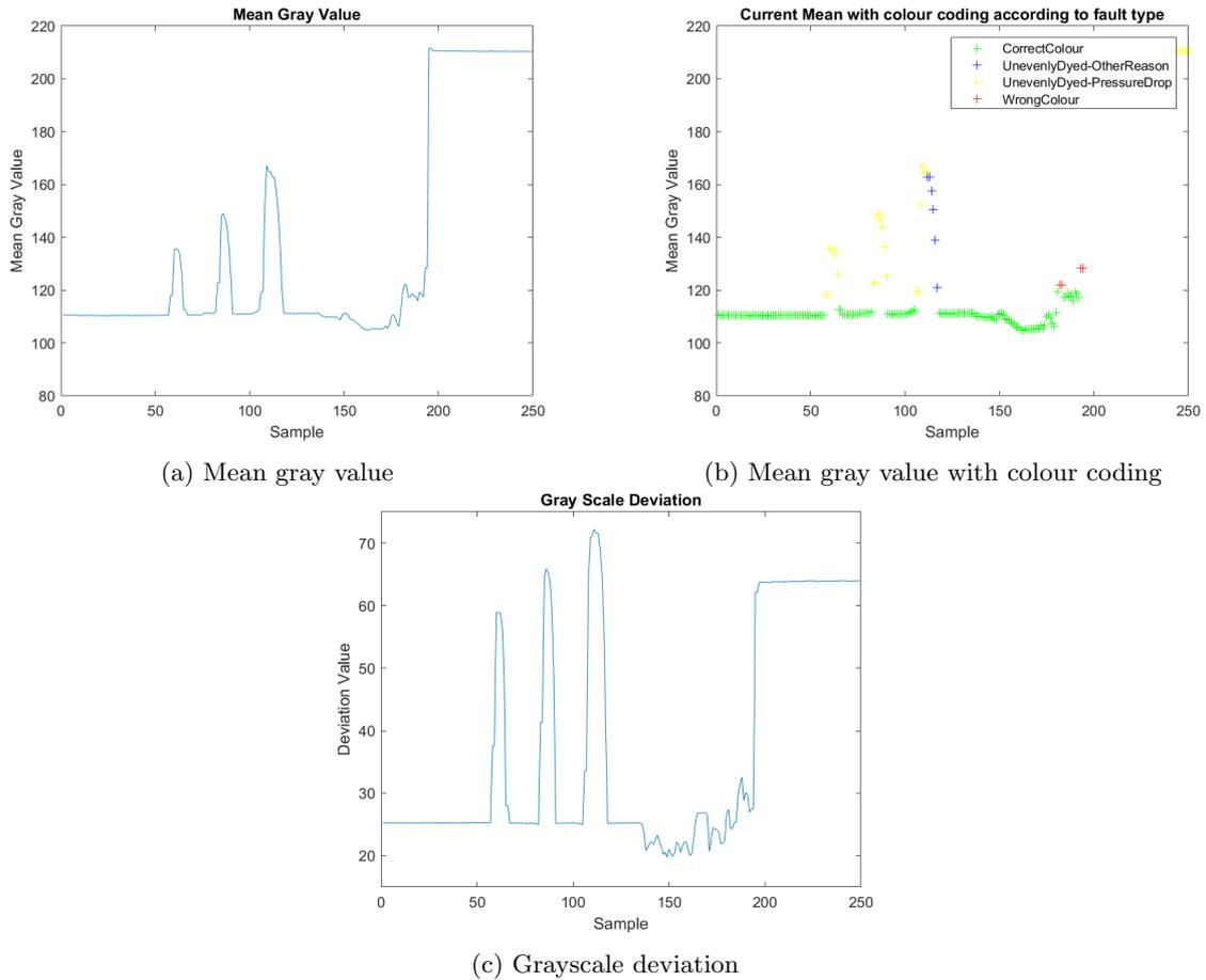
Figure 23: Captured mean and deviation, together with error message, during on site test, with moving fabric.
